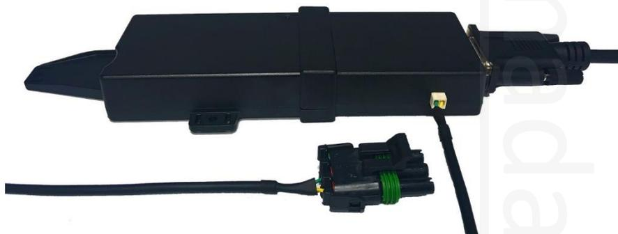
The RSA Unlock Cable is used for the unlocking of the vehicle's ECM. This cable is also required to be connected for the use of RT (Real Time) functions. This cord will be routed through the
