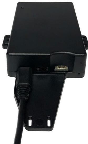
The Controller then connects to the Communication Module via a DB-15 serial connection. This is an interference fit connection. What this means is that when the two boxes are pushed together, the tight fit of the plastic cases will hold them together.
