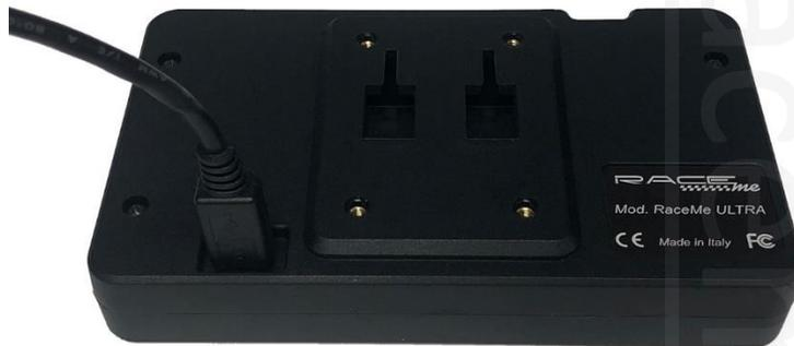
The other side of the Micro USB gets plugged into the Controller. Once again, the orientation of the cord is such that the printed “B” is facing the mounting tab, or the bottom of the controller. There are three ports in the end of the controller. The display port, shown below, the middle port (Mini USB Type B), Which can be connected to a computer for a direct relationship with our Warp custom tuning software, and the white socket, which connects to the optional EGT kit.
