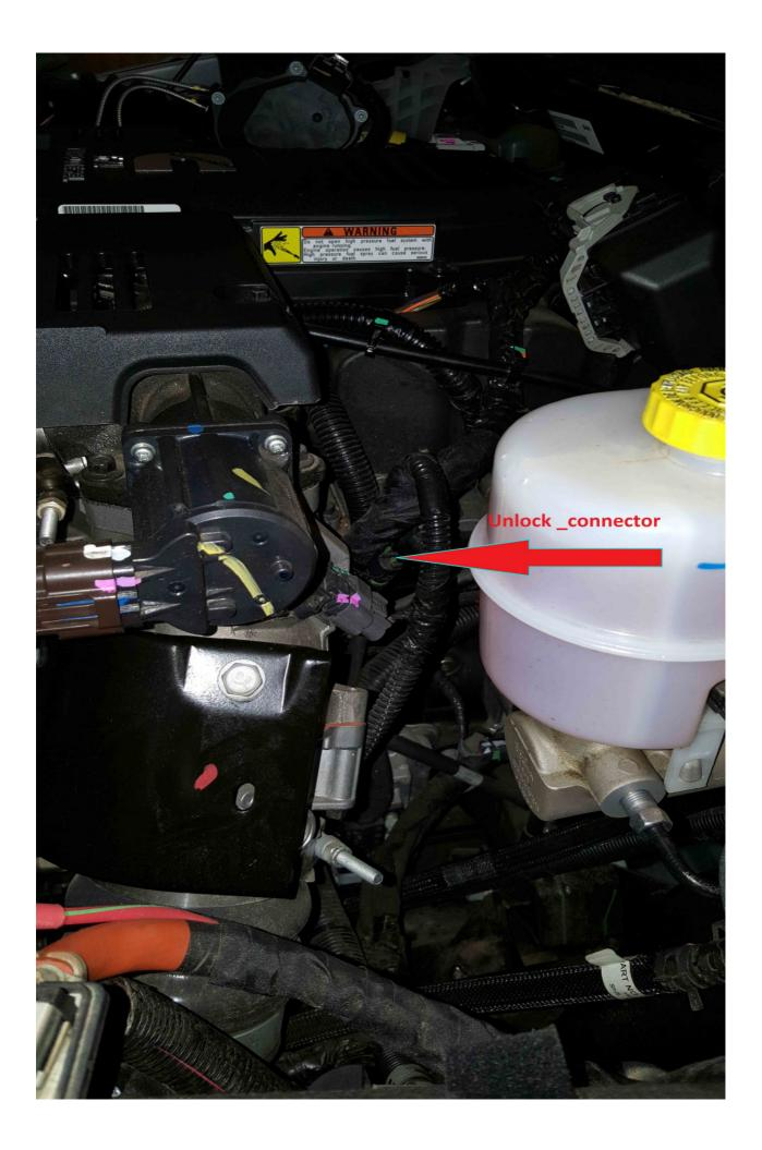
The location of this connector is not in same place on every truck! On some models you can easily locate it below the air horn (the air horn is on the driver's side of the engine, towards the front of the engine)
